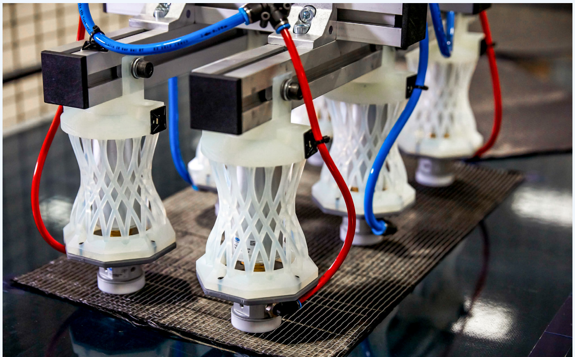
3D printed end of arm grippers, made with Formlabs Durable Resin, are used to accurately and repeatedly place carbon fiber plies as part of a composites manufacturing process.
