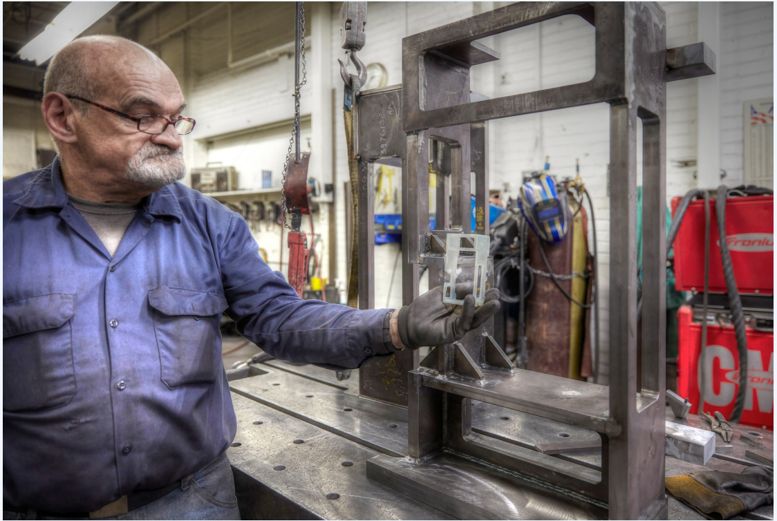
A welder at A&M Tool and Design compares a 3D printed model to the final, full-scale weldment.
